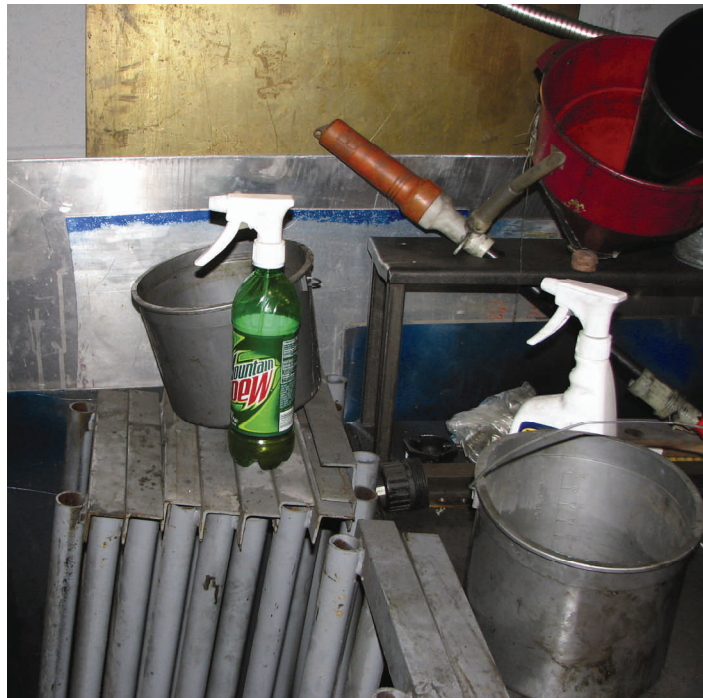
Above: Unidentified chemical(s) inside container. Per the Hazard Communication standard, chemicals shall be labeled with the identity and appropriate hazard warnings. (2007 Photo taken by IOSHA Industrial Compliance Officer, Michael Hom).
